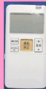
Remote controls for air conditioner
