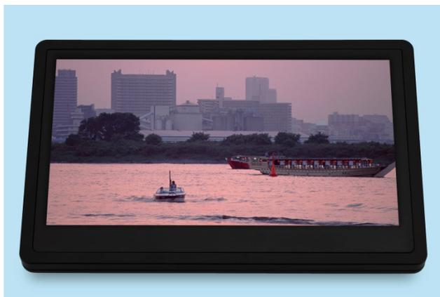
SMK Corporation has developed a capacitive touch panel consisting of double-sided ITO glass sensor “CapDuo Touch-2”, whose sensor patterns were improved from the conventional product “CapDuo Touch” to enable hybrid sensing (self-/mutual-capacitance), allowing touch detection even when a drop of water is on the panel, input when wearing gloves, and use with thick cover panel which is now in increasing demand.
