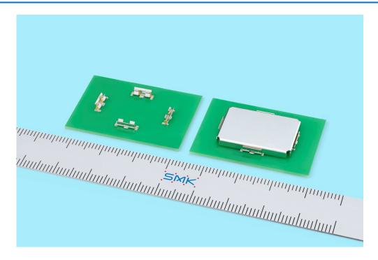
SMK Corporation has developed a shield clip mainly for automotive applications, which is used to fix noise shielding cover onto the printed circuit board (PCB). When used the clip, the shielding cover will be mounted after reflow-soldering unlike soldering the cover directly on the board, and that makes it easy to confirm solderability of the parts placed under the cover.
