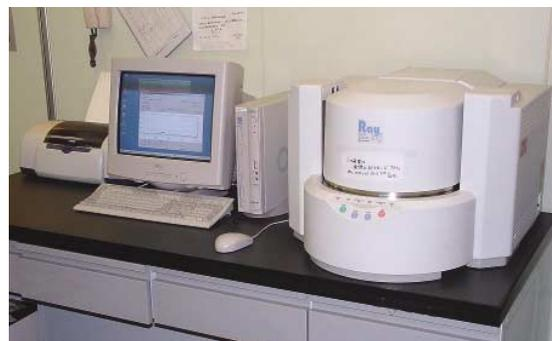
XRF spectrometer for heavy metals analysis
