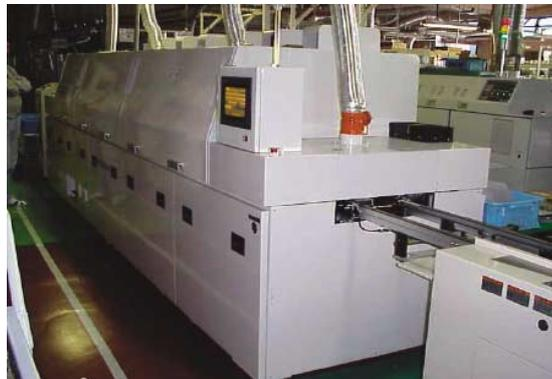
Lead-free reflow soldering machine
