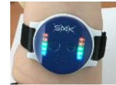
Visualization of Muscle Activity with Myoelectric Sensor (Muscle Tracker™)
